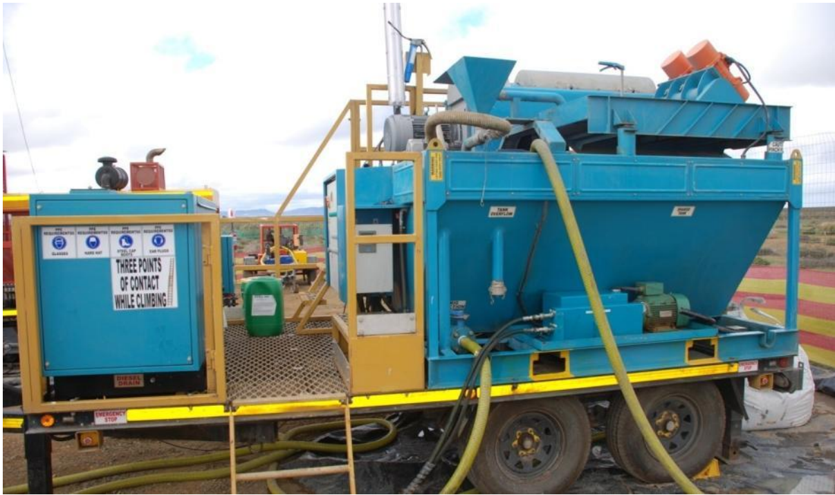
Photo 11: Sludge and drilling water from the core drill hole is circulated by pumping it to the Solid Removal Unit (SRU). The sludge and any larger particles are separated from the drill water which is re-circulated to the drill hole.
