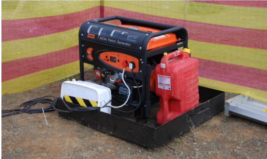
Photo 16: A drip tray is present beneath the generator in the southwestern corner of the site.
