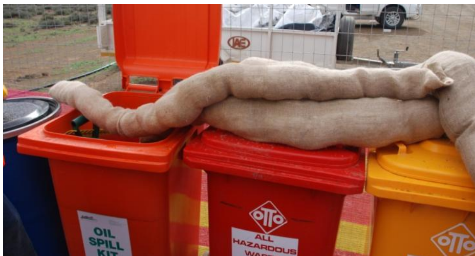
Photo 15: A petro-chemical spill kit is present on site which will be used in the event of a fuel, oil or lubricant spill. Any contaminated soil will be rehabilitated with Terrasweep and Terrafix and removed from site to Vissershok.
