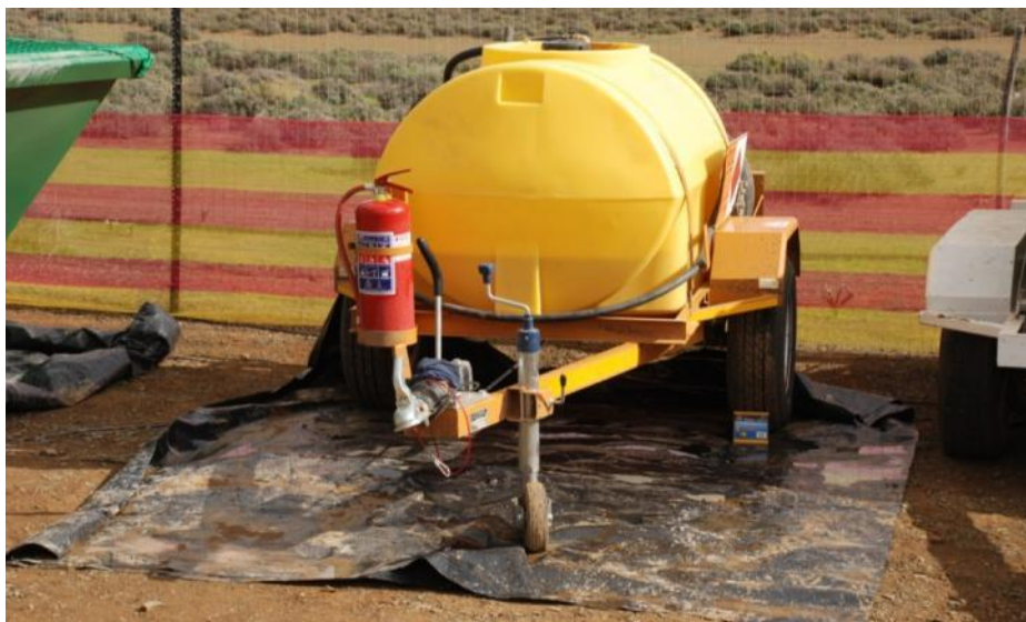
Photo 18: A mobile diesel bowser is parked on level ground (lined with plastic) and secured with tyre chocks.
