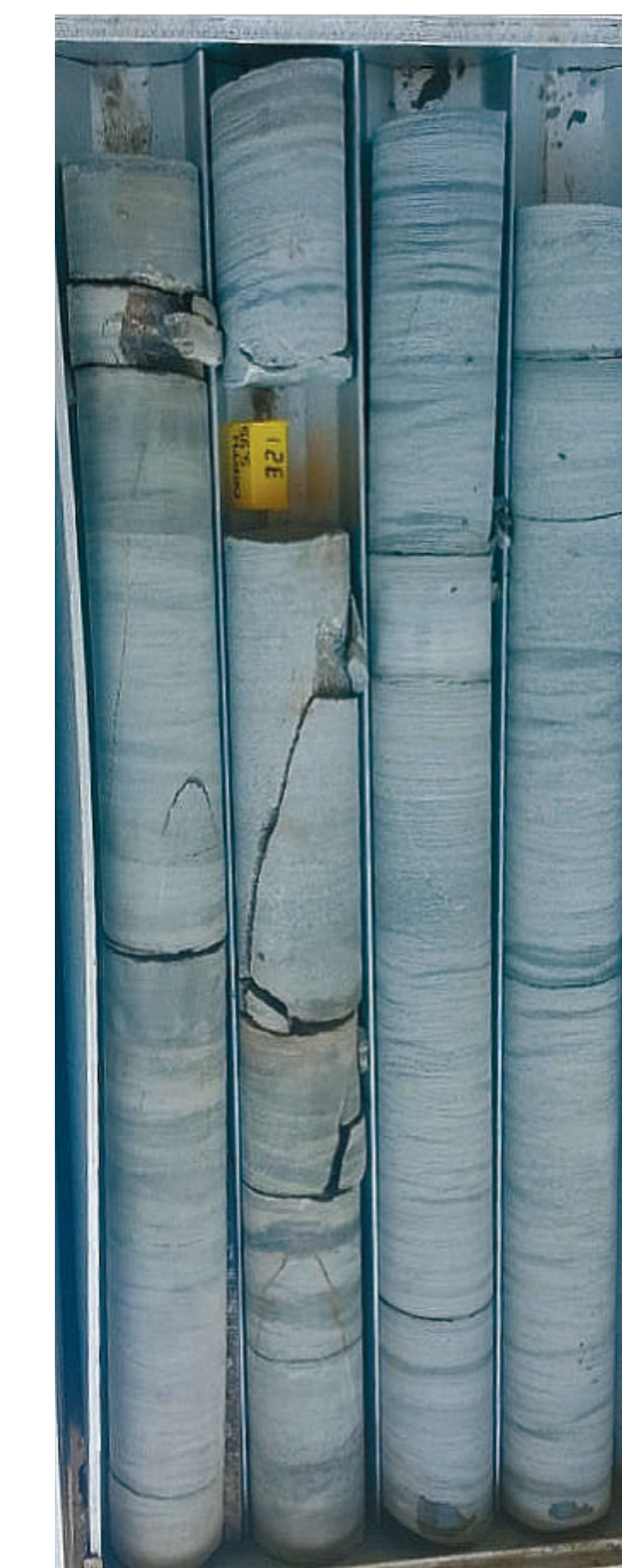
Some first drill core of Adelaide Subgroup sandstone retrieved from KVV site
