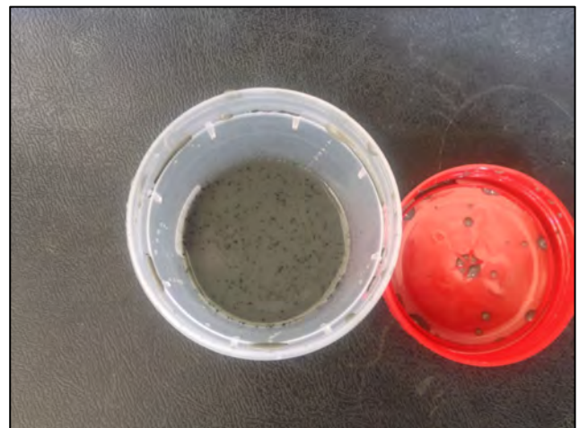
Fig. 9. Collected sample of drilling mud and diesel at a depth of 1639 m in KWV-1.
