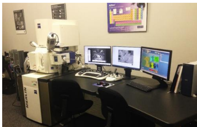
MERLIN nano-FEG SEM with EDS at SU
