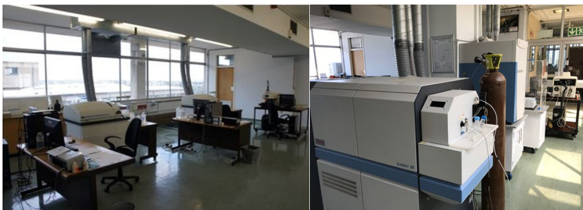
Perkin Elmer Elan DRC-e ICP-MS (left) and Thermo Element XR (right) at the Earth Lab, Wits University
