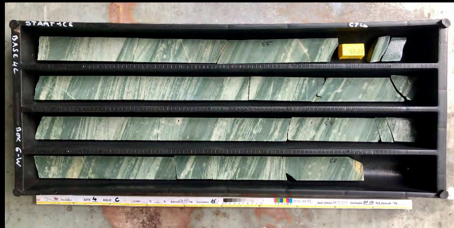
Rhythmically bedded tuffaceous-shaly sandstones
