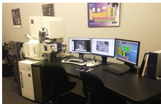
MERLIN nano-FEG SEM with EDS at SU
